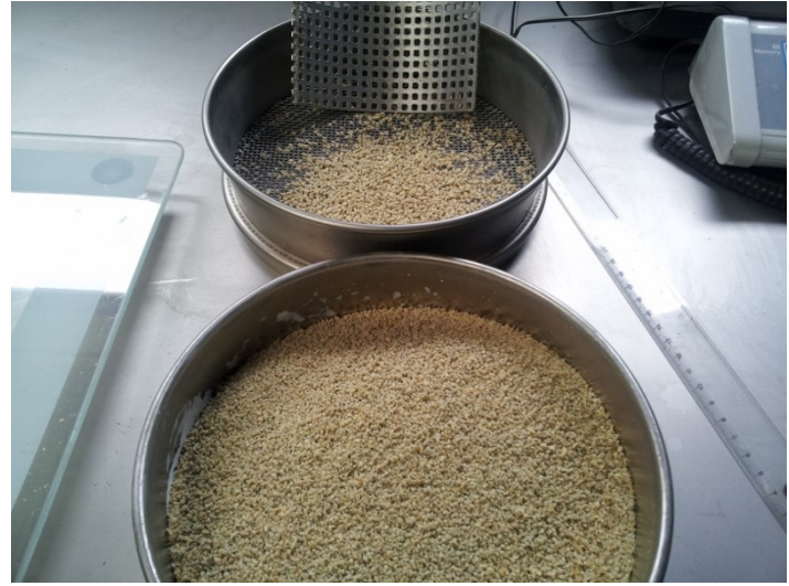
Sieved with a 2 mm sieve 90% smaller than 2 mm.
