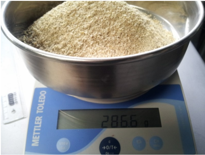
884gram Sample milled in cutting mill CM100 with 4 mm sieve and 2mm sieve.
