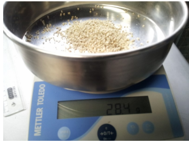
Sieved with a 2 mm sieve 90% smaller than 2 mm.
