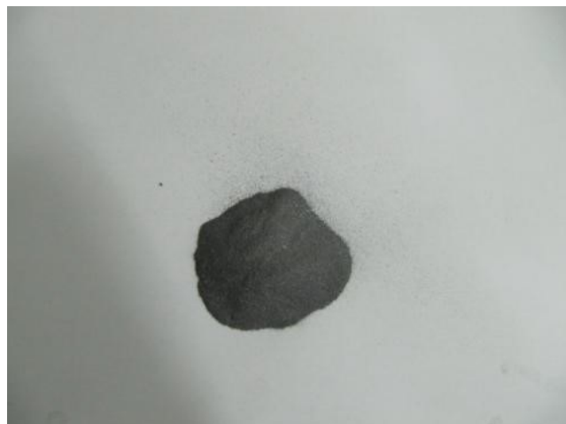
Processed sample in LM2000 after 4 minutes / Size app. 200µm
