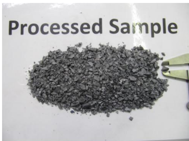
Processed Sample after 60 seconds of milling / Size app. 8 mm
