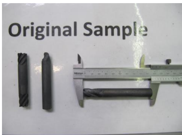
Original samples No 1. Drilling tools up to 90 mm length / weight 2,2 kgs
